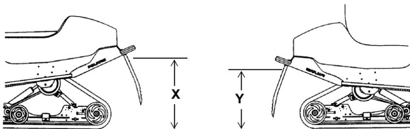
To set up the EDGE RMK rear suspension torsion spring preload, measure the distance between the ground and rear bumper (see illustration). This measurement should be taken with no rider and the rear suspension at full extension. This is measurement X.
