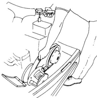
7. Locate the L-wrench in the tool kit and install it into the open threaded hole in the outer sheave of the clutch. Rotate the wrench until the sheaves open far enough to remove the belt.
