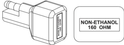
If the snowmobile is run with non-ethanol fuel be sure to install the resistor labeled “Non-Ethanol 160 OHM”. This resistor is provided in the tool kit.
