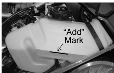
**NOTICE:** Operating the snowmobile without adequate engine lubrication can result in serious engine damage. Always check the oil level when refueling. Add oil as needed.
