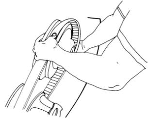
2. Rotate the L-wrench counter-clockwise to tighten the sheaves while working the belt to the outer edge of the sheaves.
