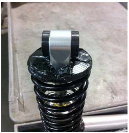
With the front track shock installed in the skid frame and the correct preload set on the coil spring, wrap duct tape around the spring, spring clip and shock shaft loop.
