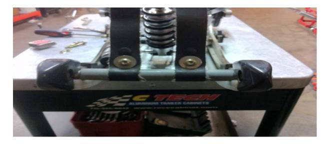
Cut 3 sections of 3/4" I.D. pvc pipe to align limiter straps. The center section should be cut to 2" long and the two outer sections to 1.5" long.
