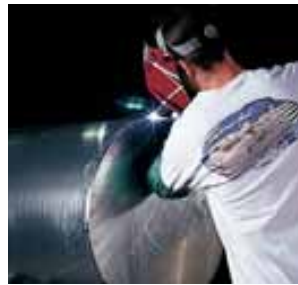
Pontoons Made of H-36 aluminum, 25 percent harder than the H-32 aluminum used by others. H-36 is more dent resistant, less prone to flex and provides maximum strength without added weight.
