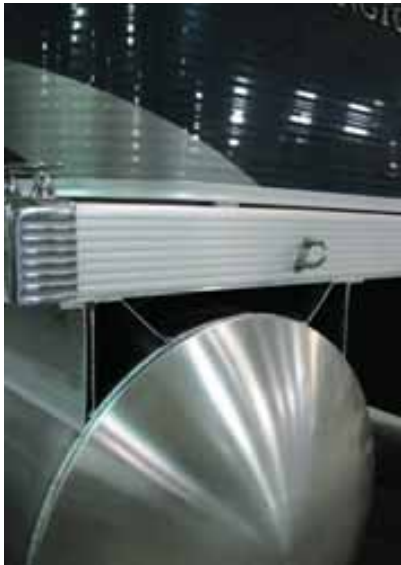
Stronger, Extruded "M" Deck Brackets Instead of the thin, bent sheet metal brackets used on other boats, Bennington uses a thick, M-shaped extrusion. Because the M-extrusion is so wide, the brackets can be spaced on 24-inch centers and still provide much better rigidity than bent sheet metal brackets on 18-inch centers.
