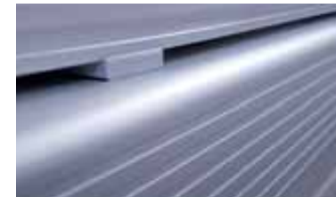
Rail Spacers for Air Flow .25-inch rail spacers between the deck and rail allow easy deck drainage and the added ventilation reduces mold and mildew when your boat is covered.
