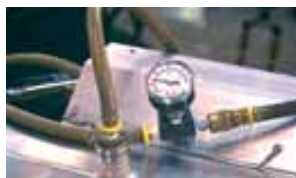
Pressure-Tested Pontoons Bennington pontoons are made with multiple chambers with valves and separate headers. Each chamber is pressure tested twice.
