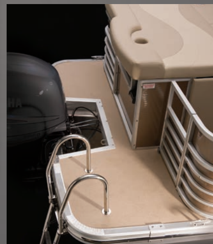
Extended Aft Deck with Tuff-Ply® Vinyl Flooring and Telescoping Boarding Ladder (optional)
