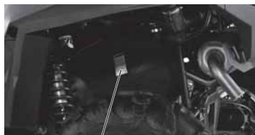
Belt Debris Warning
