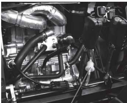
Fuel Tank Vent Filter
