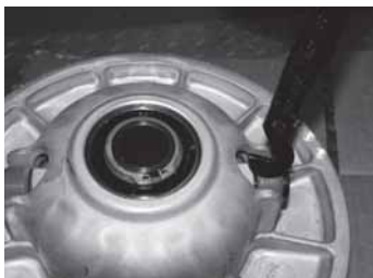
Insert hooked end of tool.
